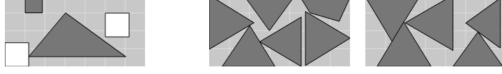
Fig. 1. The distance condition (2)(3) requires that each square of the background grid has to be at least partially covered. Left: A feasible one-bin layout for two tiles (grey) with two support plates (white). Right: An optimal solution using two bins without support plates (instance 3 in Table 1).
